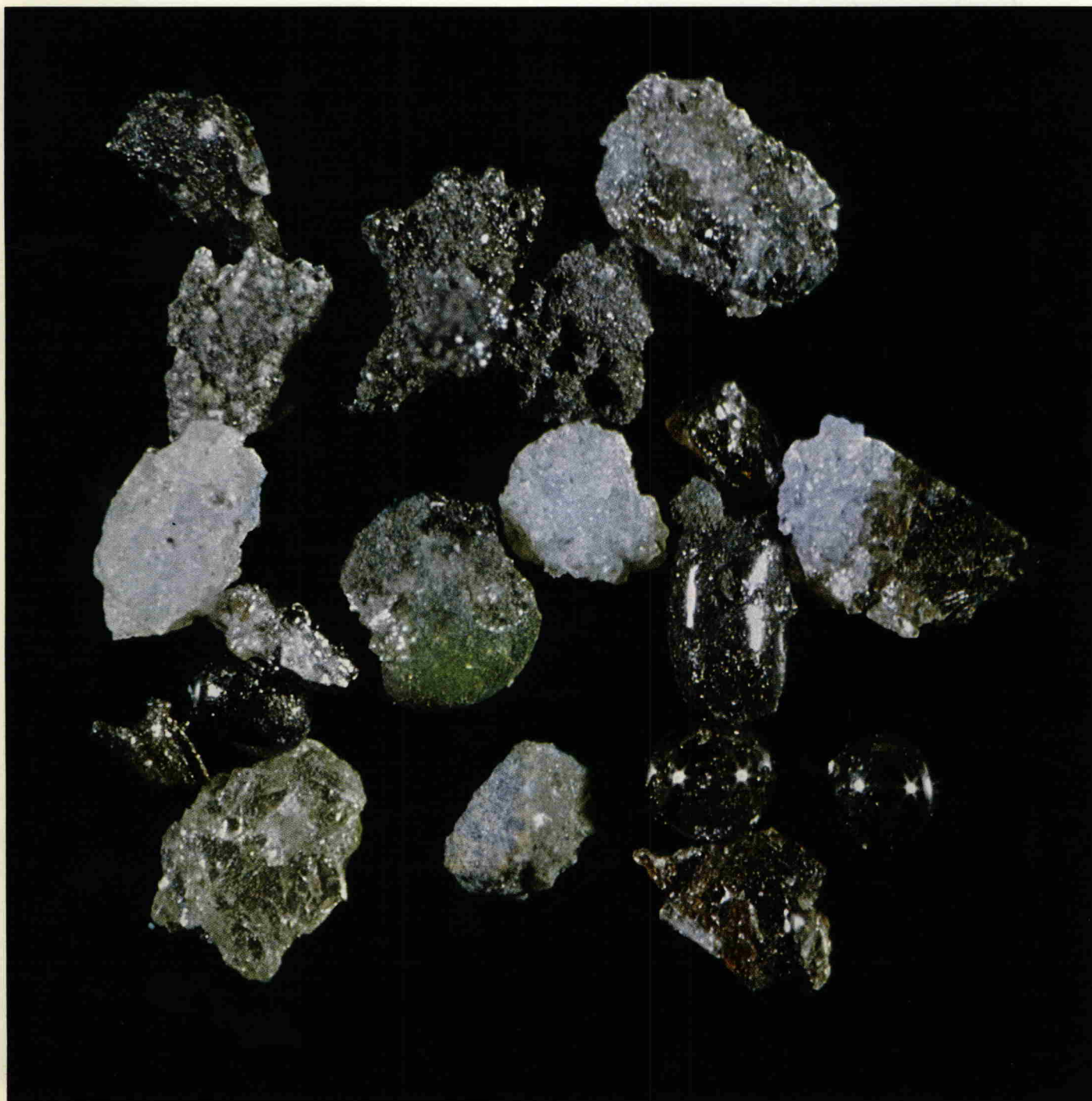
Apollo 11. Fragments of lunar rocks and minerals. Size \frac{1}{4} - \frac{1}{2} mm ZEISS Tessovar.
